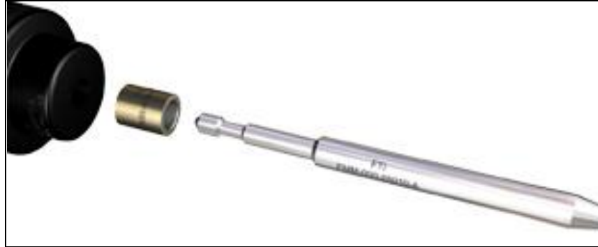
2. Place bushing on mandrel and insert into puller
