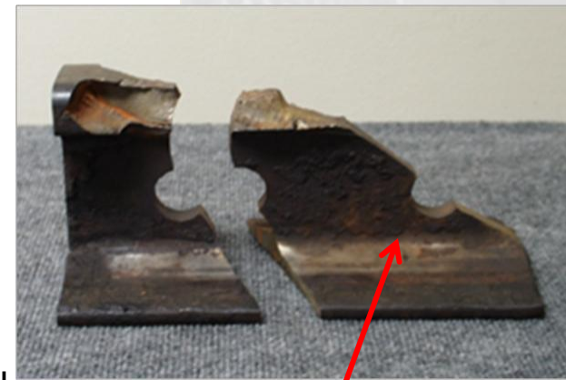
Typical rail-end bolt hole fatigue failure
